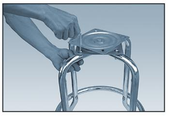
STEP 3 Place swivel on top of legs & align holes. With top plate at a 45° angle to the other, insert large bolts and screw on lock nuts securely. If swivel is tight, place on a carpeted floor, stand on it and twist - you should be able to turn it smoothly.
